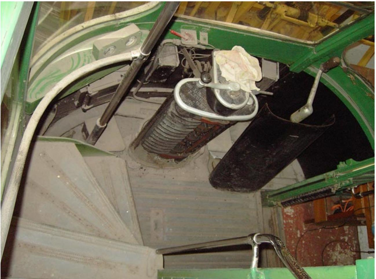
**The windscreen from 'A' end was stripped out and rebuilt, incorporating new parts to replace those too worn or rusted to re-use. New toughened glass was fitted to the lower section to replace a broken original. New windscreen wiper motors were sourced and parts from them incorporated into the original air operated motor wipers which were completely stripped down and rebuilt.**
